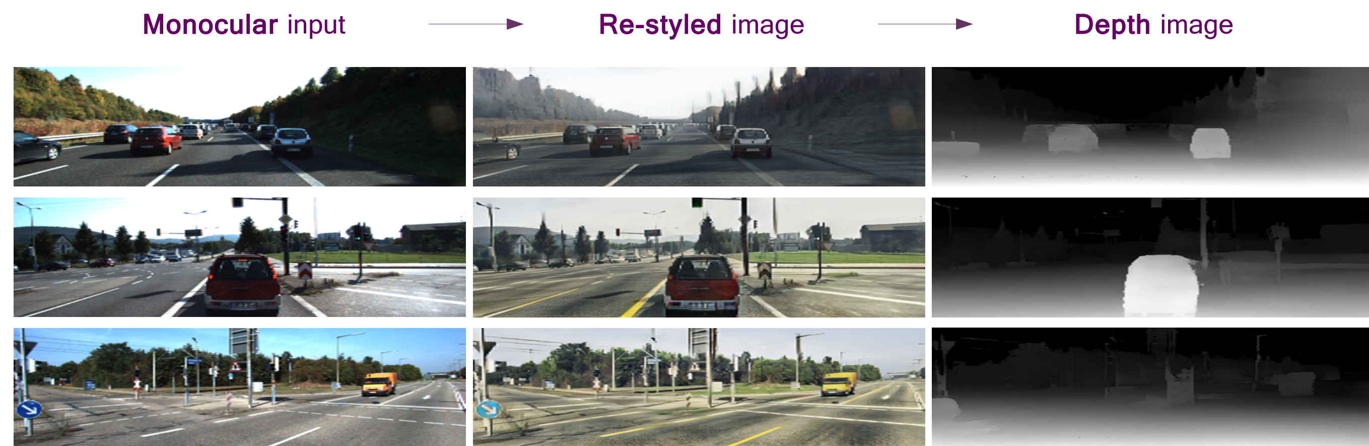
Monocular depth estimation model trained on synthetic data produces sharp and plausible depth when applied to real-world images transformed to the style of synthetic images.
