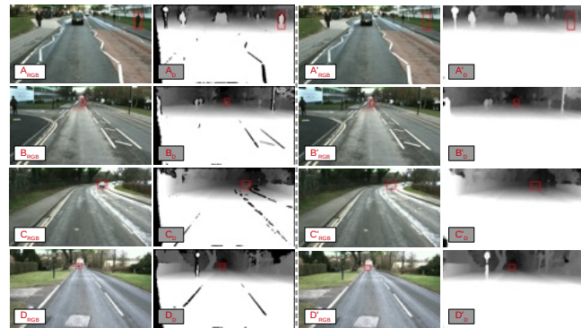
Applied to automotive stereo disparity maps to remove dynamic scene objects (vehicles, pedestrians) - original (left), filled (right).
