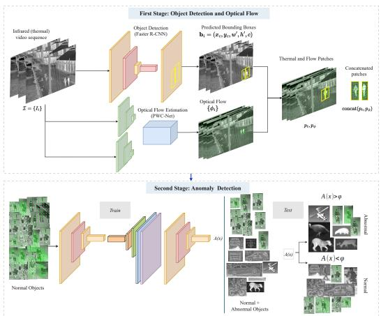
Figure 2. The proposed architecture for anomaly detection.
