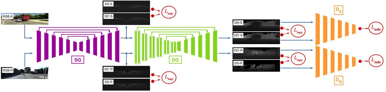
Figure 2: Overall training procedure of the approach. **S**: synthetic data from the virtual environment [17]; **R**: data captured from the real world [54]; **SD**: sparse depth; **DD**: dense depth; **SG**: sparse generator network; **DG**: dense generator network.
