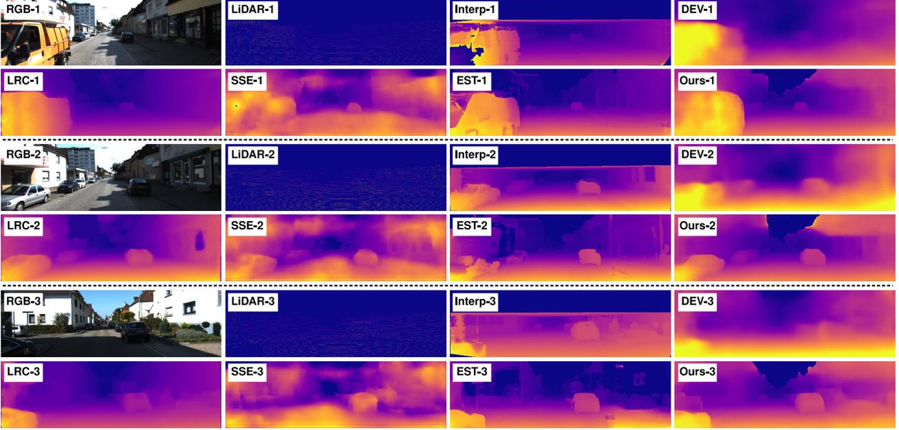
Figure 3: Comparing the results of our monocular depth estimation approach against [5, 20, 31, 66]. Adjusted disparity images are included for better visibility. **RGB**: input colour image; **DEV**: depth and ego-motion from video [66]; **LRC**: left-right consistency [20]; **SSE**: semi-supervised estimation [31]; **EST**: estimation via style transfer [5].
