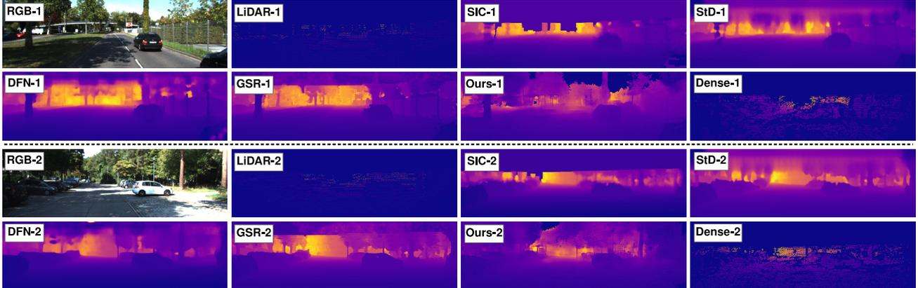
Figure 5: Comparing our depth completion results against [15, 40, 54, 50]. The depth images have been adjusted for better visualization. **RGB**: input colour image; **LiDAR**: sparse depth input; **SIC**: sparsity invariant CNN [54]; **StD**: sparse to dense completion [40]; **DFN**: deep fusion network [50]; **GSR**: guided sparse regression [15]; **Dense**: dense ground truth from [54].
